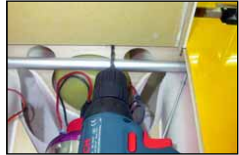
(above) Drill a 8mm Ø hole thru' the rear bulkhead for the thrust vector linkage as shown.
