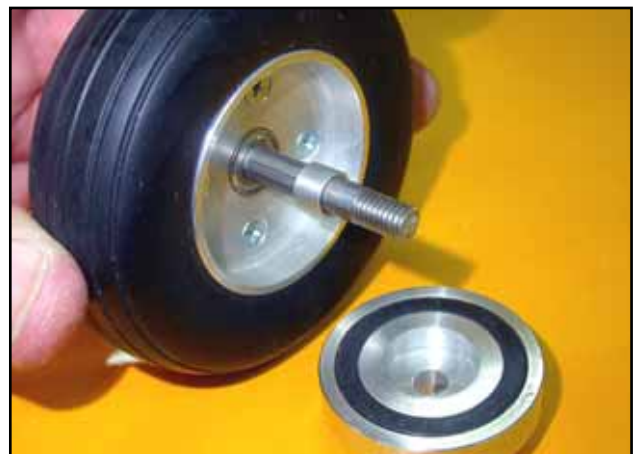
(above) Don't forget to install the short aluminium tubes between the wheel and brake drum.
