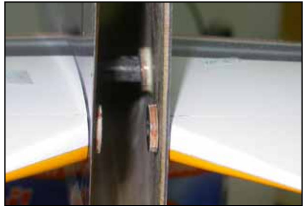
Stab spar tube and reinforcement rings
